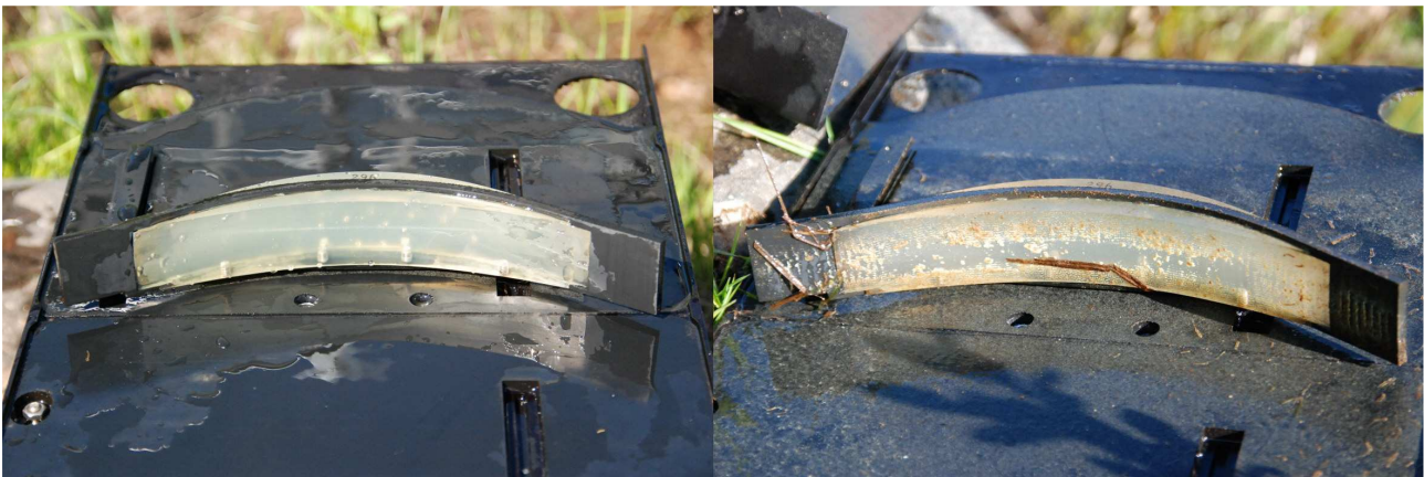
Figure 32. A clean (left) and pollen covered lens (right).
